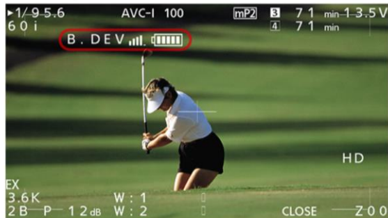
Image: Viewfinder Displays of the Connection Conditions (marked red)
