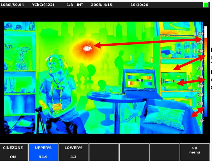
Luminance signal is displayed with color. The distribution of the luminance signal within the picture can be checked easily
