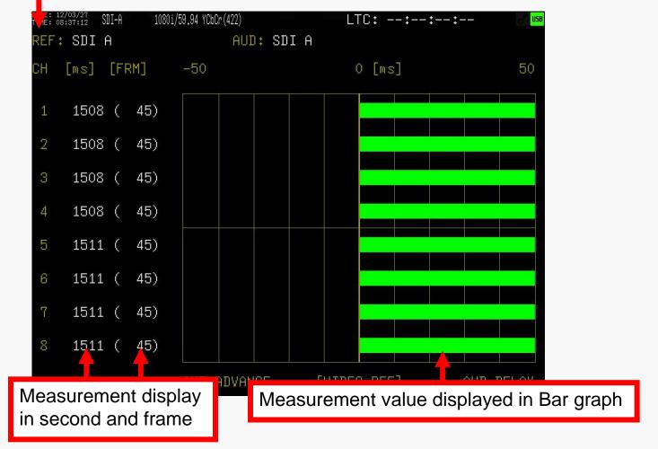
Lip-Sync auto measurement screen, 8ch audio simultaneous measurement is possible
